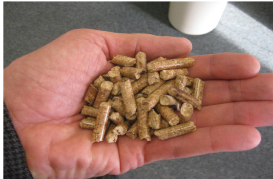
Randy is holding a handful of wood pellets used for the biogasoline process.
